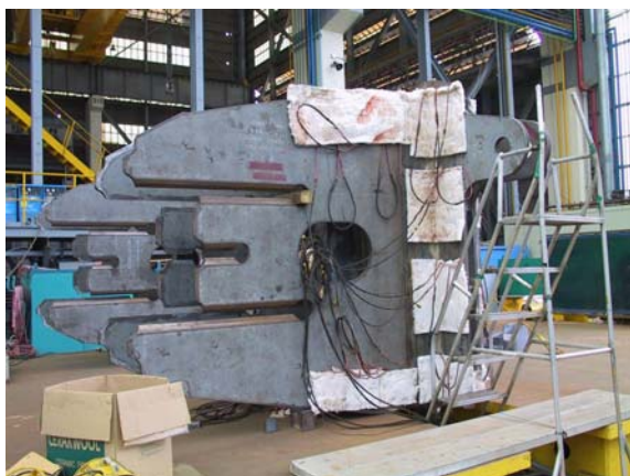
Figure 14: Construction and assembly of skid box and skidding systems
