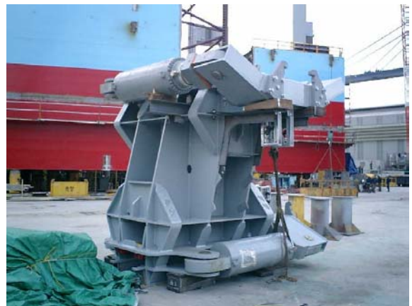
Figure 14: Construction and assembly of skid box and skidding systems
