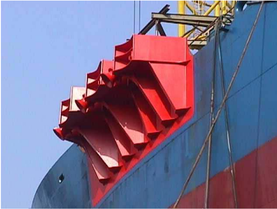
Figure 9 - Integration Spread Moored System
