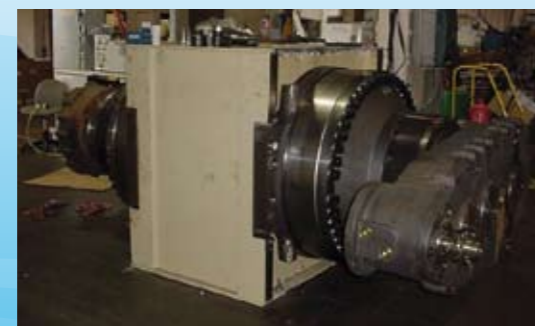
Test of 2 jacking units in back-to-back configuration
