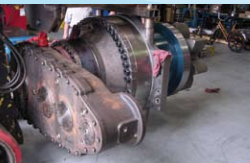
As-built jacking unit (before painting)
