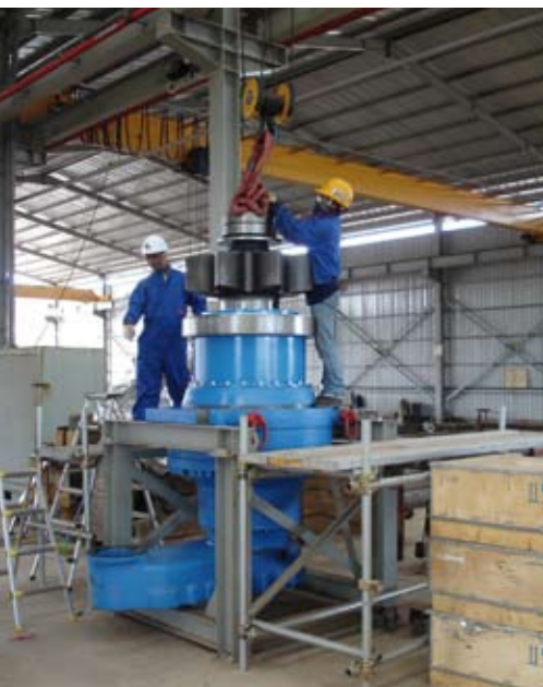
Assembly pinion onto gearbox
